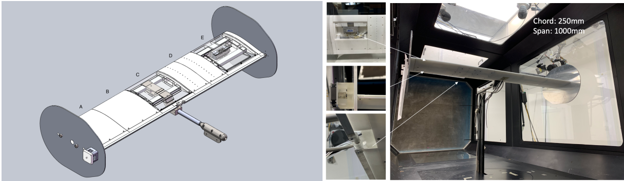
Fig. 2 Setup. Left: CAD rendition of the test wing. The flow is from left to right. The wing is made from five interchangeable 3D-printed segments, labelled A-E, each 200 mm in width, and mounted onto two rectangular aluminum spars that span the entire wing from tip to tip. The overall span to the model is 1000 mm (exclude the endplate and outside structure). The center segment (C) holds a steel mounting bracket which clamps over the wing spars and connects to the sting, which itself is integrated with an internal six-axis force/torque transducer. In the configuration shown on the right end (E) holds the Scanivalve pressure transducer, while segment D has pressure taps for surface pressure measurements. Right: The model is installed in the wind tunnel, mounting on a pitch-yaw mechanism. The motor to control the Gurney flap can be seen on the outside of the left-side endplate. The driving and supporting mechanisms are also shown in the figures.
